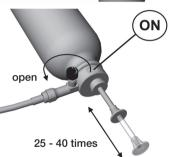
The air pressure in the fuel bottle is crucial to the heat of the stove. When preparing food, you may have to do some more pumping in order to maintain maximum heat. However, if you pump up too high a pressure the fuel flow will be too great resulting in a yellow flame.
