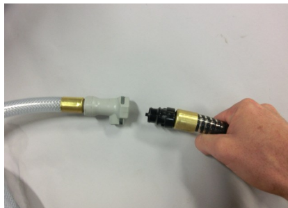
Attaching intake service hose to hose to sea strainer.
