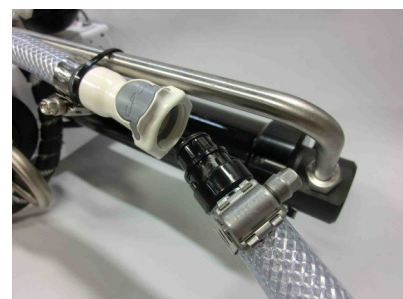
Connecting brine discharge service hose
